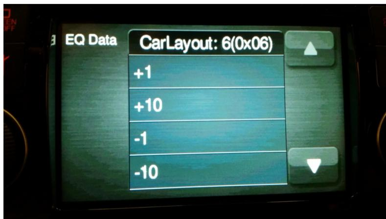
6. Touch the line for **+1** or **-1** to scroll through the different layouts until the desired layout appears in the top line. For enabling rear speakers, select **8(0x08)**.
