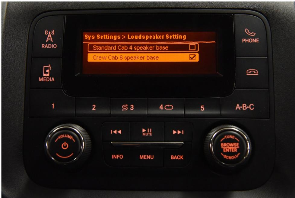
9. Exit the Engineering Mode menu by pressing the **Back** button 3 times.
