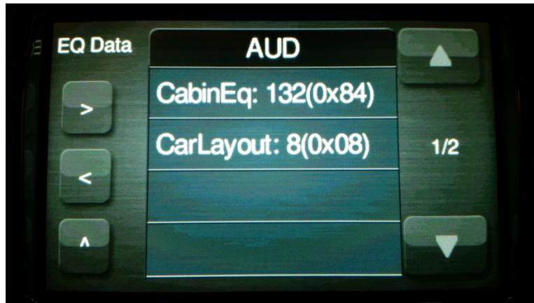
9. Exit the **AUD** screen by touching the small **UP ARROW** (^) button located to the left of the menu. The following screen will appear.
