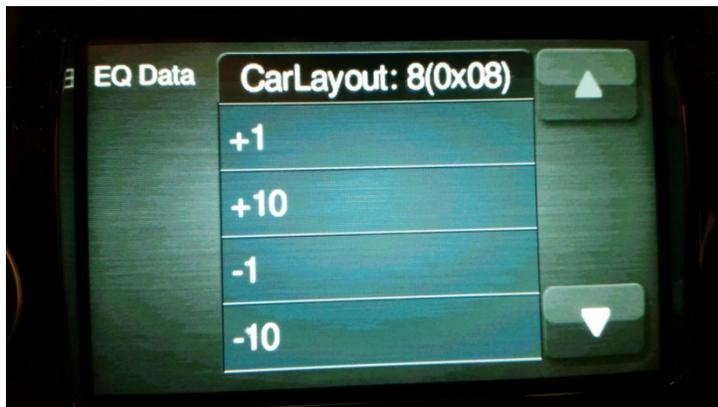
7. Touch the **UP** and **DOWN** arrow soft buttons on the screen to locate the lines for **OK** and **CANCEL**.
